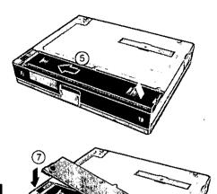
(5) Slide the battery pack inward until it is firmly in place.
